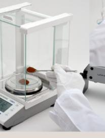
We have considerably reduced stabilization time by improved filtering technology. Short stabilization time is indispensable for efficient weighing operation.
