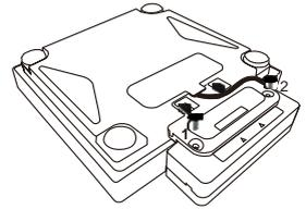
2. Open the signal cable box cover as arrow.
