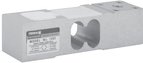
Model 1242 is a high accuracy, low profile, low cost, two beam, single point load cell ideally suited for industrial application where space is limited. Typical applications include platforms, hanging scales and personal weighers.
