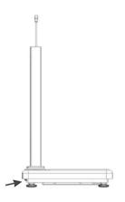
4. Load cell signal cable go through the indicator holder.
