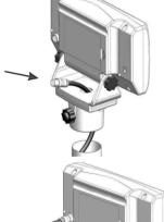
5. Connect indicator cable and fasten the fixed knob.
