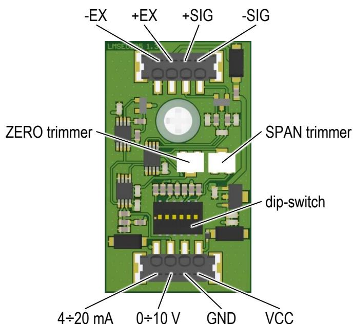
The terminals take cables with a cross-section between 0.2 and 0.5 mm<sup>2</sup>.
